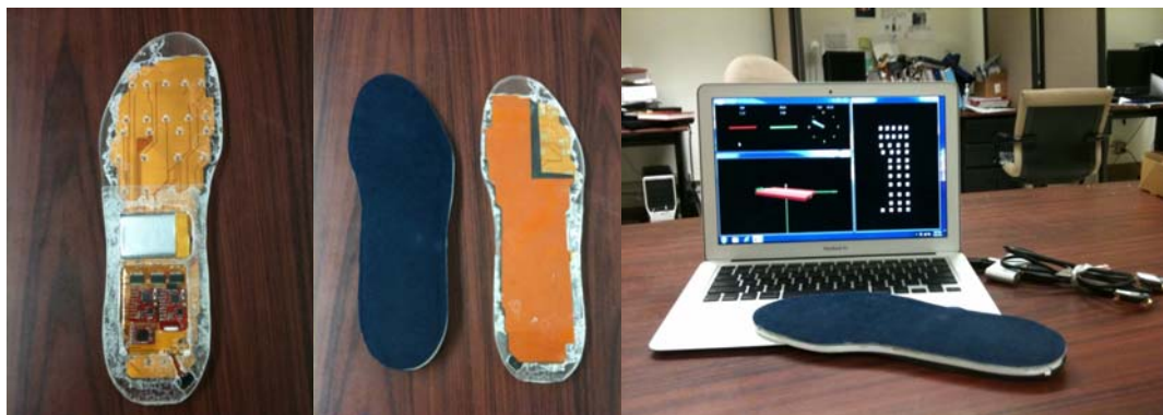
Figure 3: (a) Insole Circuit Structure (b) Smart Insole in Packaging (c) Smart Insole in Demo
