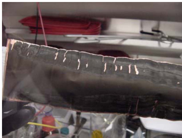
Figure 10. (Color online) Images of (bottom) negative and (top) positive tapes during destructive physical analysis of cell B. The positive tape appears to be pristine, while the negative tape shows clear signs of delamination near the edge of the tape.
