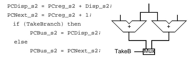
• Explicitly defining the intermediate signals help determine the position of the MUX.
