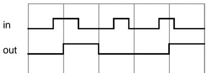
Delay control is used most commonly for clock or pattern generation;
