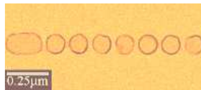
Fig. 6. An MQCA chain with the elongated input dot on the left hand side.
