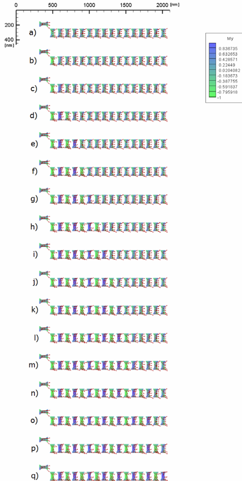
Figure 9.2 Simulated relaxation of an antiferromagnetically-coupled chain of nanomagnets shows as the switching propagates in time from (a) to (q) along the chain.
