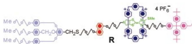
FIG. 1. (Color) Molecular structure of the bistable [2]rotaxane R used to form LB monolayers. The molecule has a hydrophobic (dark green) and a hydrophilic (light blue) stopper. The [2]rotaxane has cyclobis(paraquat- p -phenylene) (dark blue) as the ring component and the supporting counterions are hexafluorophosphate.
