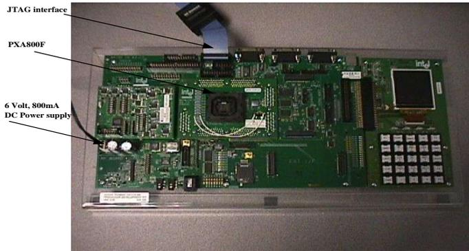
**Figure 1: The Intel® PXA800F Processor Evaluation board**
