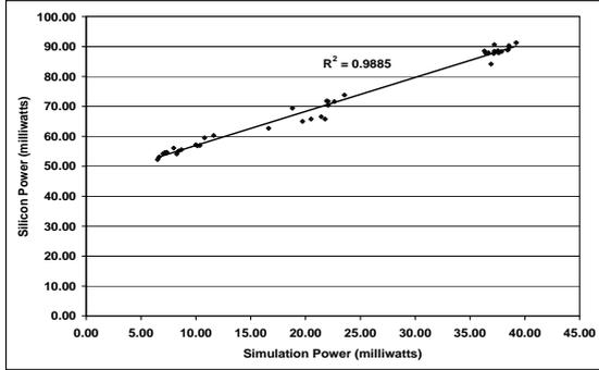
Figure 6: Power  $P_{totmax}$  Correlation for Data Processing Components (no differencing)
