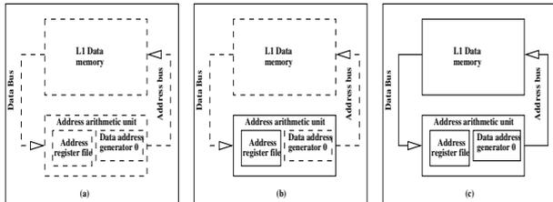
Figure 5: (a) Base (b) Minimal (c) Maximal Switching Cases of the Data Load Circuitry
