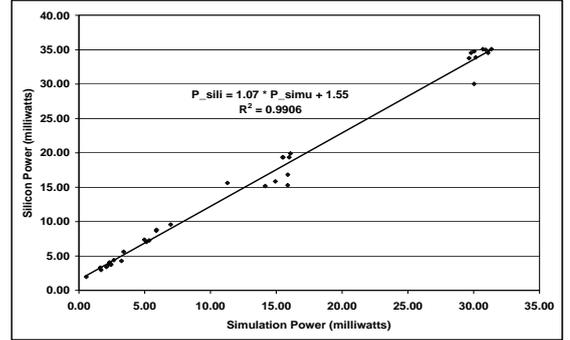
Figure 7: Power  $P_{switch}$  Correlation for Data Processing Components (differencing)
