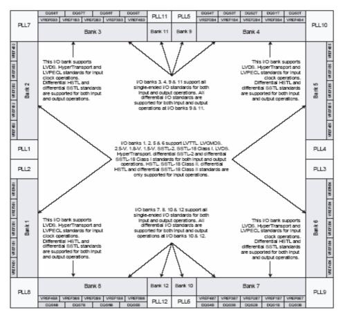
Each I/O bank has its own VCCIO pins. A single device can support 1.5-, 1.8-, 2.5-, and 3.3-V interfaces; each bank can support a different VCCIO level independently. Each bank also has dedicated VREF pins to support the voltage-referenced standards (such as SSTL-2).
