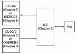
All Virtex-4 FPGAs have configurable high-performance SelectIO drivers and receivers, supporting a wide variety of standard interfaces. The robust feature set includes programmable control of output strength and slew rate, and on-chip termination using Digitally Controlled Impedance (DCI). All banks can support 3.3V I/O.
