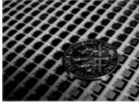
Fig.1 Photograph of batch-fabricated bandpass filters on a single panel; each block represents a filter
