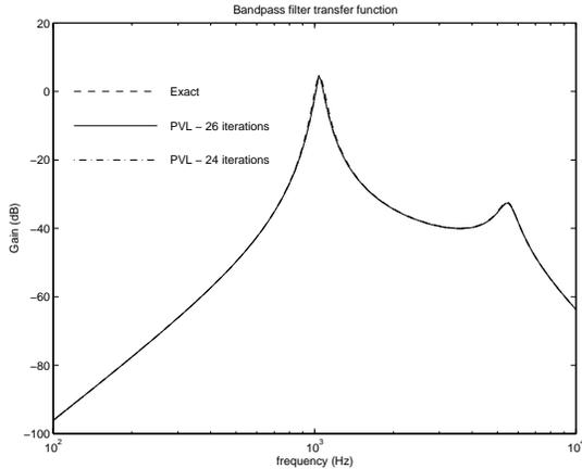
Figure 5: Bandpass filter transfer characteristic
