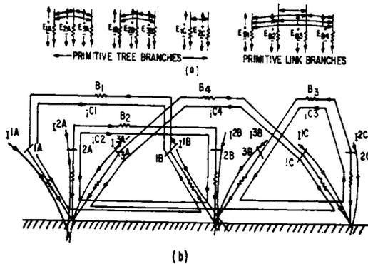
Fig. 8. (a) Newly created primitive network. (b) Network equivalent of original network.
