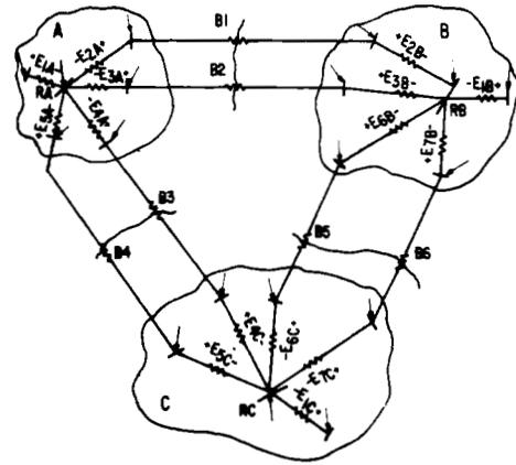
Fig. 9. Equivalent representation of subdivisions, torn subdivisions not attached (r). (RA, RB, RC represent reference buses.)
