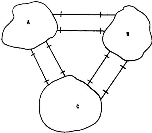
Fig. 2. Example of interconnected power system consisting of three power companies (A, B, C).
