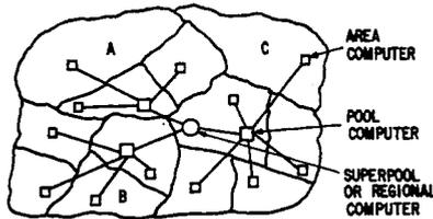
Fig. 15. Diagrammatic example of a multicomputer configuration formed by a three-pool region (A, B, and C), with area subdivisions within each pool.
