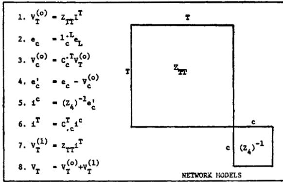
For the example case in Fig. 8(b), where all subdivisions emanate from a common reference,  $C_c^T$  simply assigns signs to currents  $i_c'$  as seen from the example case in Fig. 8(b).
