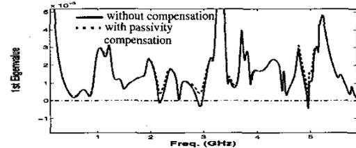
Fig. 4. Eigenvalue v/s freq. of  $Re(Y(s))$  - with compensation
