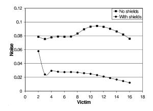
Figure 2: Noise in a sixteen-bit  $1000\mu$ m-long bus. The driver size is  $200\times$ , and the wire spacing is  $0.6\mu$ m
