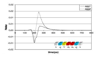
Figure 3: noises on the victim caused by two aggressors in a five-bit  $1000\mu m$ -long bus. The driver size is  $30\times$ , and the wire spacing is  $1.7\mu m$ .
