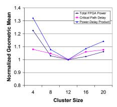
Figure 16 Total FPGA power, critical path delay and power-delay product v.s. cluster size (routing\_fullbuf2, LUT Size = 4)
