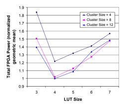
Figure 15 Total FPGA power for three cluster sizes (routing fullbuf2)
