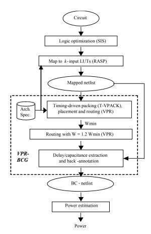
Figure 10 Power Evaluation Framework (fpgaEva-LP)
