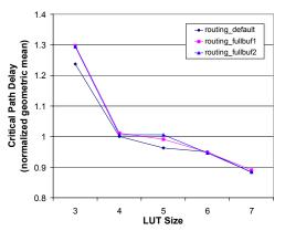
Figure 13 Critical path delay for three routing architectures (Cluster Size = 4)
