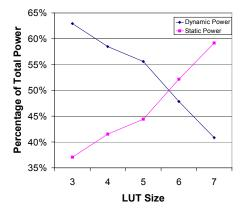
Figure 19 Breakdown of total power: dynamic power and static power (Cluster Size = 12)
