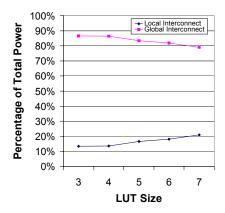
Figure 18 Breakdown of interconnect power (Cluster Size = 12)
