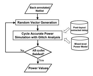
Figure 9 Overall Power Calculation
