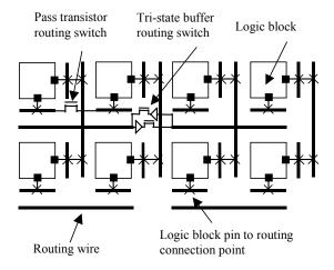
Figure 3 An Island-style Routing Architecture
