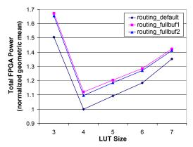
Figure 12 Total FPGA power for three routing architectures (Cluster Size = 4)
