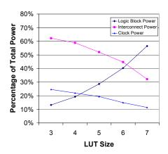
Figure 17 Breakdown of total power: logic block power, interconnect power and clock power (Cluster Size = 12)
