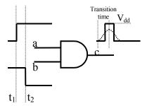
Figure 7 Glitches at a Circuit Node.
