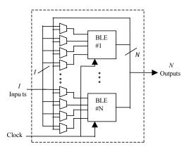
Figure 2 Cluster-based Logic Block
