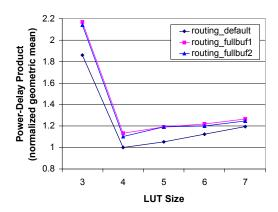
Figure 14 Power-delay product for three routing architectures (Cluster Size = 4)
