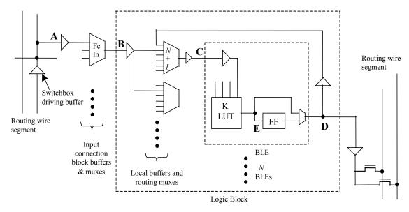
Figure 5 Schematic for Logic Block
