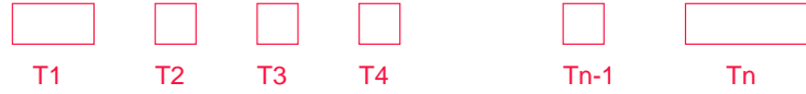
Figure 7.1: The cross-section view for a block of n traces, where T_1 and T_n are dedicated power/ground traces. The widths for the traces are W_1, W_2, \dots , and W_n , respectively. The spacings between them are S_1, S_2, \dots and S_{n-1} , respectively.
