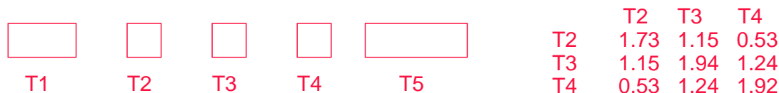
Figure 7.2: Loop inductance ( nH ) by specifying that T_1 and T_5 are current return paths.
