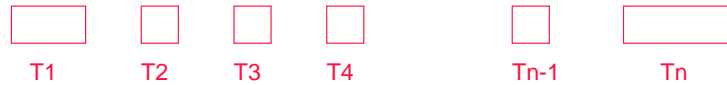
Figure 2: The cross-section view for a block of n traces, where T_1 and T_n are dedicated power/ground traces. The widths for the traces are W_1, W_2, \dots , and W_n , respectively. The spacings between them are S_1, S_2, \dots and S_{n-1} , respectively.
