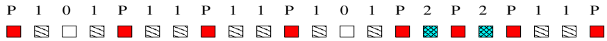
Fig. 2. A valid track assignment solution with a minimum number of power nets ( p_t = 3 ).
