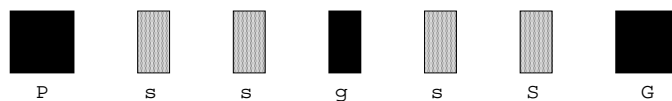
Fig. 1. A cross-sectional view of a coplanar interconnect structure with a shield inserted.
