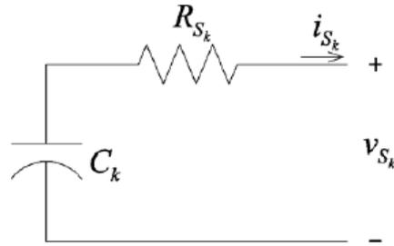
Fig 3 Super Capacitor Equivalent Circuit
