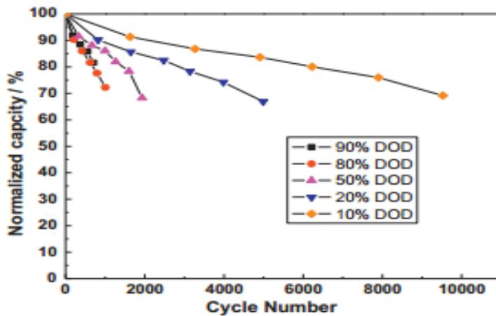
Fig 2 Battery Cycle Life VS DOD
