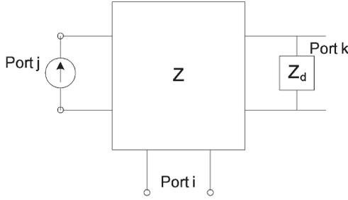
Fig. 3. Inserting one decoupling capacitor.
