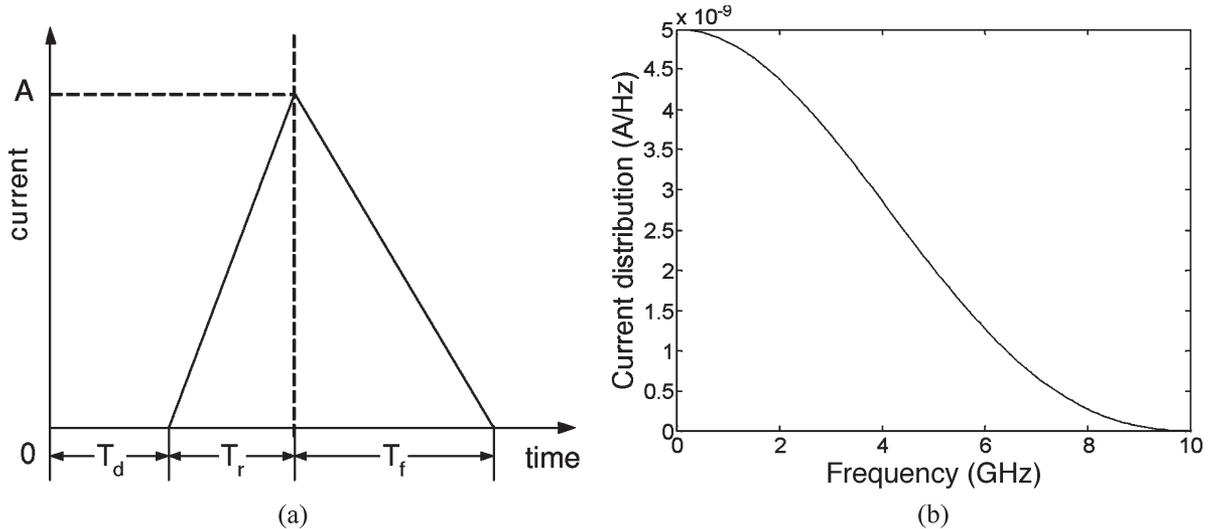
Fig. 2. Switching current model. (a) Time-domain waveform. (b) Spectrum.
