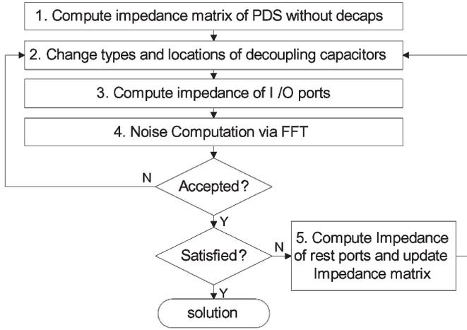
Fig. 4. Efficient decoupling capacitor optimization flow.
