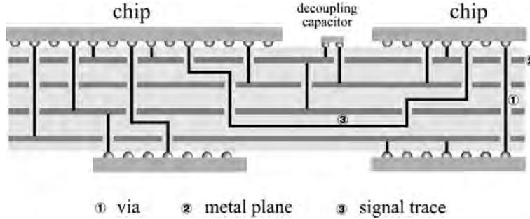
Fig. 3.17 Resistive, capacitive, and inductive parasitics of a package [17].
