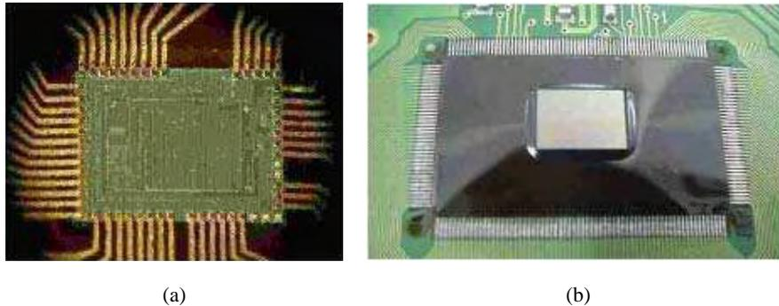
Fig. 2.5 (a) Inner lead bonds and (b) outer lead bonds [89].
