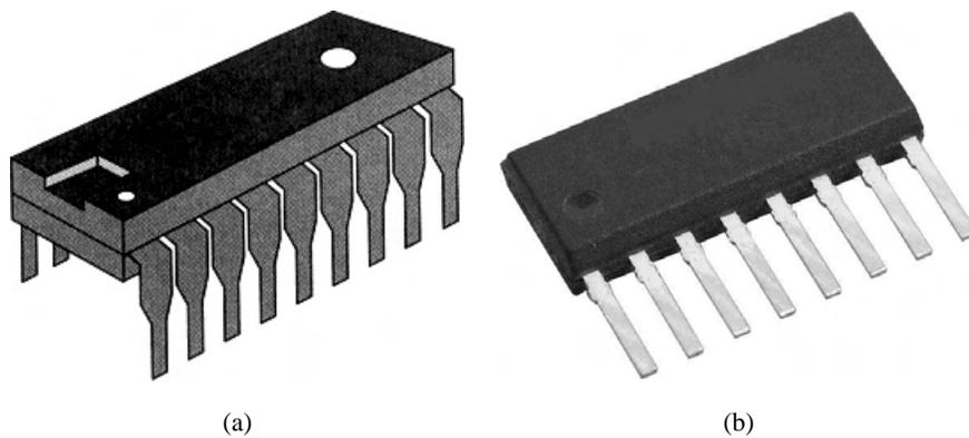
Fig. 2.11 (a) Dual-in-line package and (b) Single-in-line package [5].
