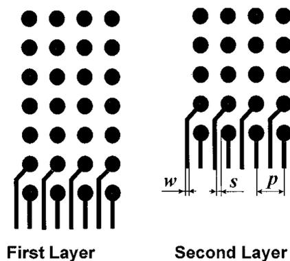
Fig. 4.2 Typical conventional routing structure on first and second layers.
