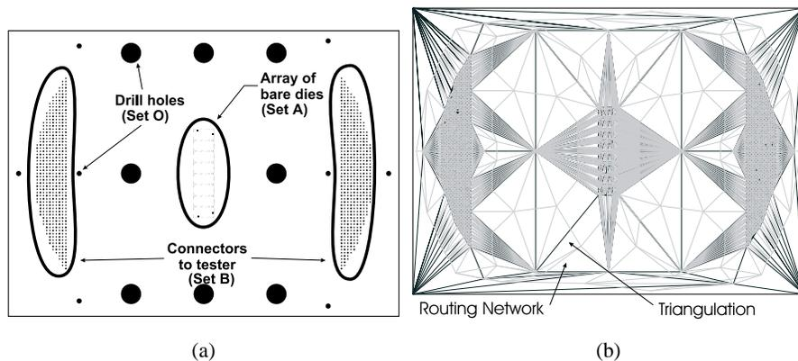
Fig. 4.9 (a) An unrouted example: each pad in the center must be connected to one pad on the edge connector, and (b) the triangulated routing network of the (a).
