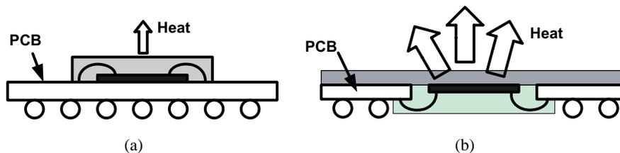
Fig. 2.8 (a) Cavity up and (b) Cavity down wire bond substrate [33].
