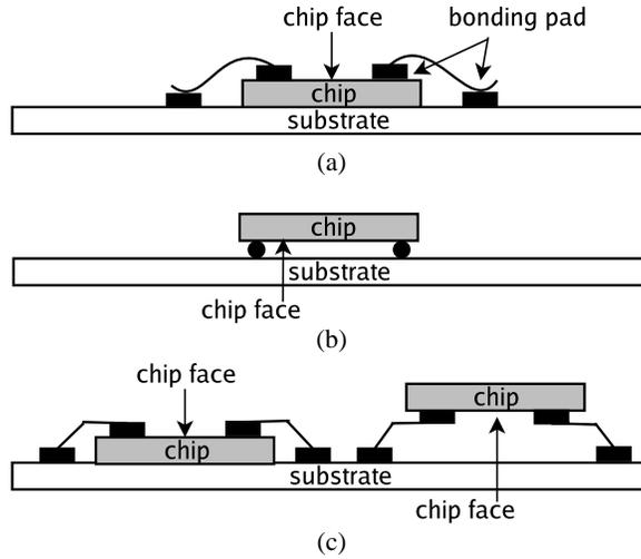
Fig. 2.2 Illustrations of (a) wire, (b) flip chip, and (c) tape-automated bonding [5].
