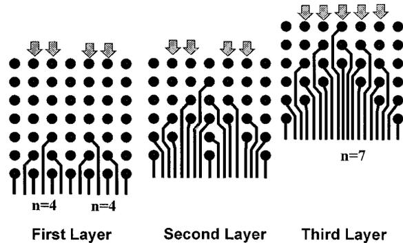
Fig. 4.5 An arrangement of the hybrid channels with  $n = 7$ .
