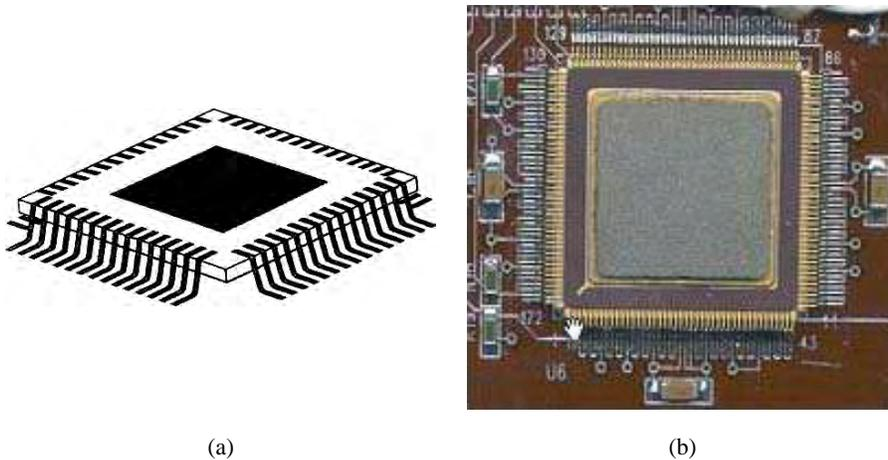
Fig. 2.14 Quad flat package [5].
