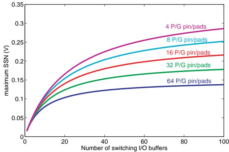
Fig. 3.16 Relationship between SSN and the number of switching I/O buffers for different numbers of power/ground pins/pads.
