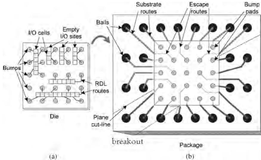
Fig. 4.1 I/O placement and package routing phases for flip chip design.
