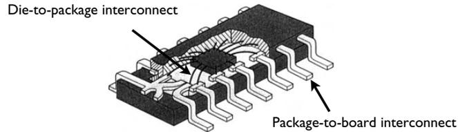
Fig. 2.1 Elements of a semiconductor package [5].
