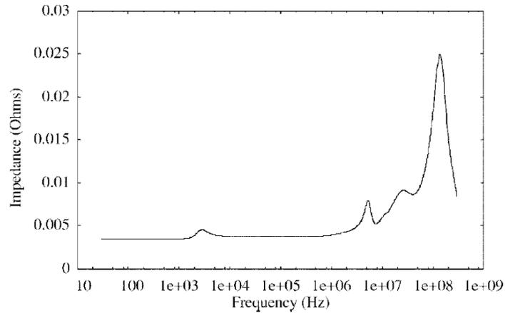
Fig. 3.13 PDS impedance seen from the chip [7].
