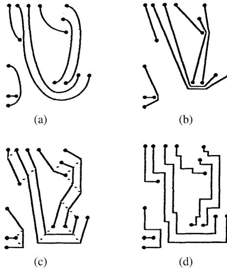
Fig. 4.11 Rubber-band sketch-based detailed routing.
