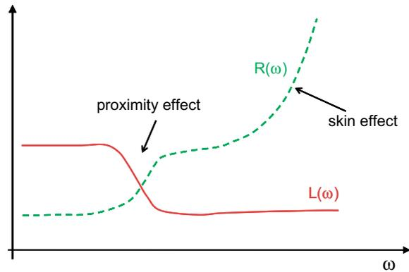
Fig. 3.8 Frequency dependence of package resistance and inductance.
