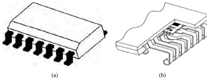
Fig. 2.13 Small outline package with (a) gull wing leads and (b) J-bend leads [5].
