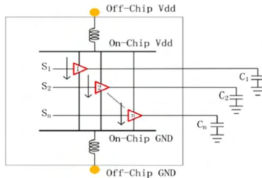
Fig. 3.14 SSN caused by the simultaneous switching of I/O buffers.
