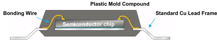
Fig. 2.6 Illustration of lead-frame-based plastic package [10].
