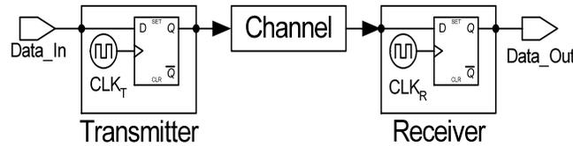
Fig. 3.2 Block diagram of a chip-to-chip communication channel. The main components are the transmitter, the receiver, and the lossy channel that is composed of the RDL routes, the package traces, and the PCB traces.
