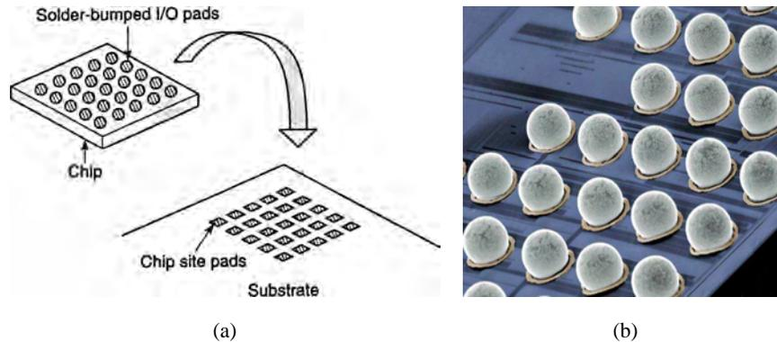
Fig. 2.4 (a) Flip chip bonding and (b) a fabrication example [33].
