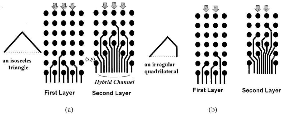
Fig. 4.4 Examples of preferential routing with hybrid channels: (a)  $n = 5$  and (b)  $n = 4$ .
