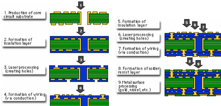
Fig. 2.9 Manufacturing process for multi-layer organic build-up substrate [88].
