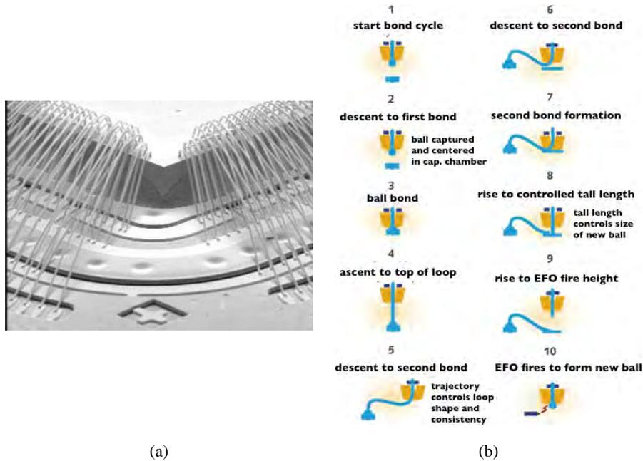
Fig. 2.3 (a) Example of wire bonding and (b) wire bonding (ball bond) steps [68].
