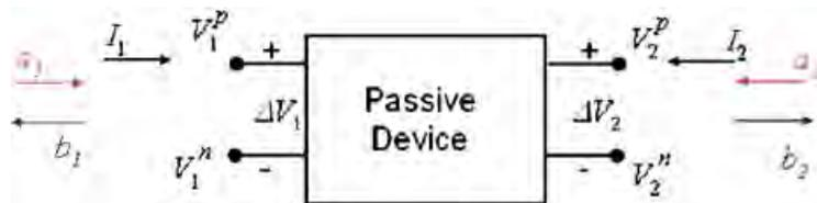
Fig. 3.11 Illustration of voltages and power waves for a two-port system.
