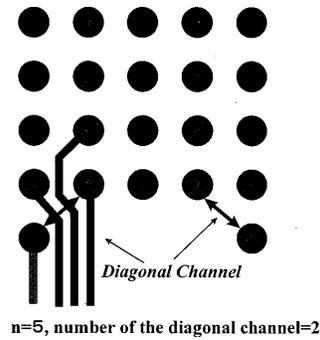
Fig. 4.3 Illustration of hybrid channels.
