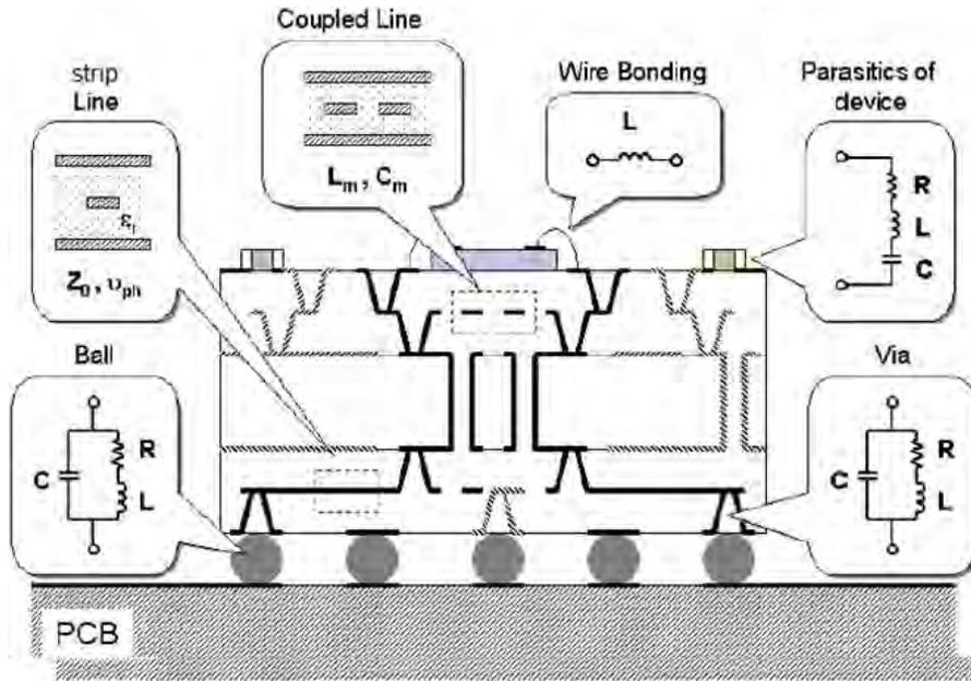
Fig. 3.7 Resistive, capacitive, and inductive parasitics of a package [87].
