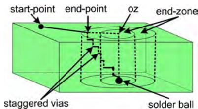
Fig. 4.10 Illustration of staggered vias.
