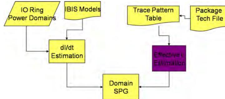
Fig. 3.3 Quick simultaneous switching noise estimation model that uses the IBIS models of the drivers, the package layer parameters, and the trace model of the signal routes from the driver to the package pins.
