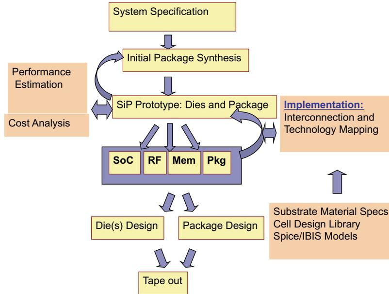
Fig. 3.1 A coherent SiP design methodology.
