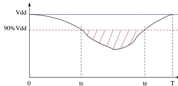
Fig. 3.18 Illustration of voltage drop with the shaded area showing the metric (tolerance bound = 90%  $V_{dd}$ ).
