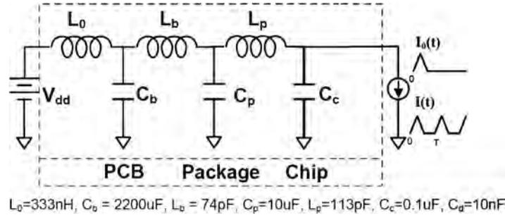
Fig. 3.12 Illustration of power delivery system.
