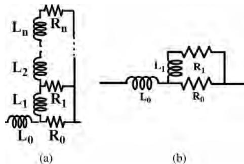
Fig. 3.10 RL ladder circuit to model frequency dependence.
