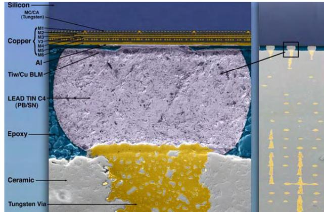
Fig. 2.10 Cross-section of ceramic substrate [33].
