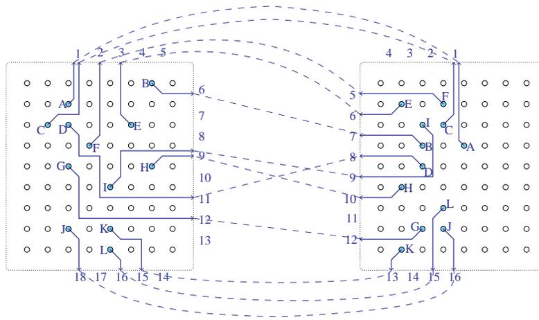
Fig. 4.8 An escape routing solution for 12 nets. The escape slots are identified on the boundaries of components. The connections in the intermediate area are shown by dashed lines.
