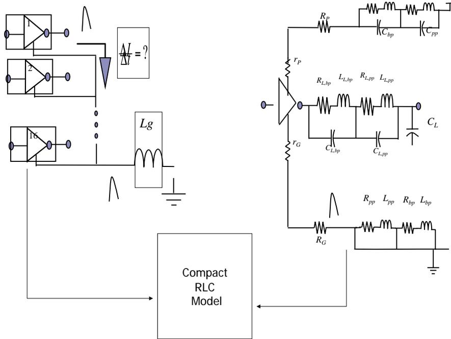
Fig. 3.6 RLC model for estimating the noise and timing of the signal interface early in the SiP design stage.
