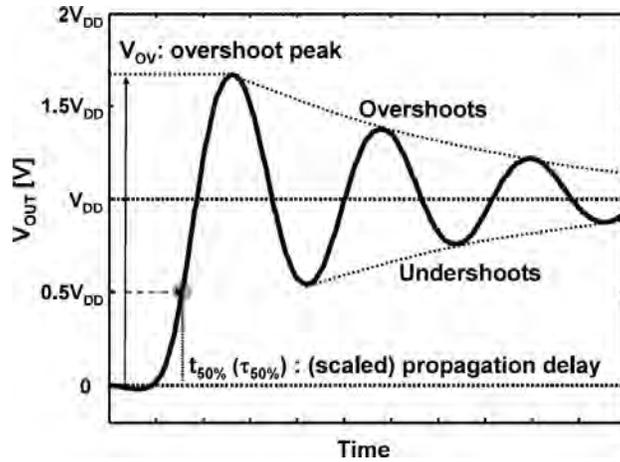
Fig. 3.9 Overshoot, ring back, and propagation delay caused by inductive effect [2].
