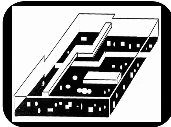
Fig. 3.5 The picture on the right shows a poor voltage domain partitioning in the package. The perforated plane does not provide a stable reference and causes a large inductance loop and noise problems in the package.
