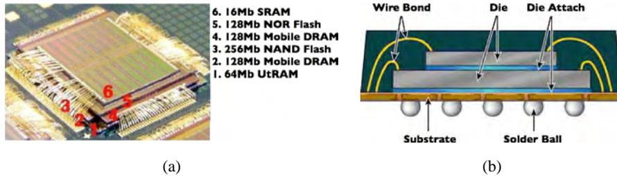
Fig. 2.17 (a) System in package example and (b) 3D stacking [5].
