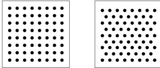
Fig. 4.6 Square grid array *versus* hexagonal grid array.
