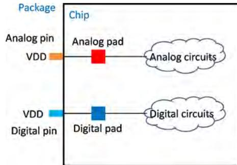
Fig. 3.15 Separation of digital and analog power/ground pads.
