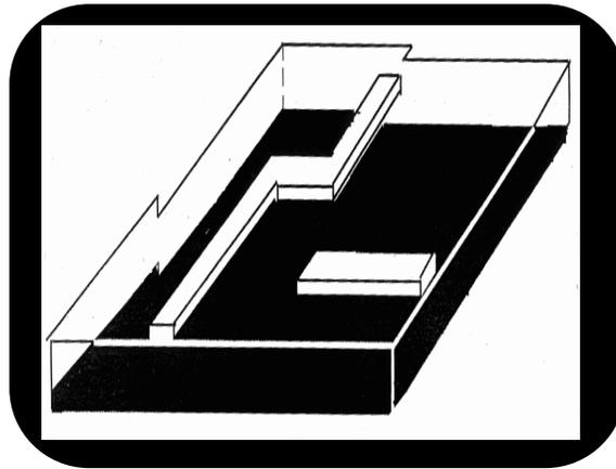
Fig. 3.4 This picture shows a solid plane that provides a stable reference for the traces above and below it. This design provides a tighter return path loop, which renders the effective loop inductance smaller.
