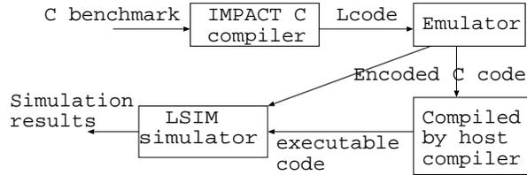
Figure 1.1. Flow diagram for IMPACT
