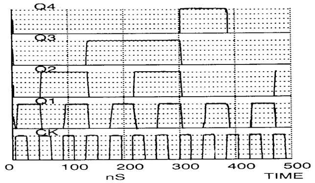
Figure 4 Waveforms in 10-bit Counter
