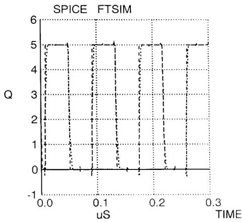
Figure 2 Waveform Comparison Between FTSIM & SPICE
