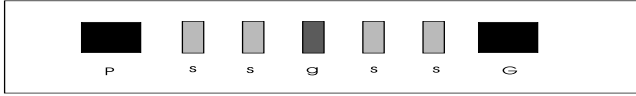
Figure 1. A cross-section view of a coplanar interconnect structure with a shield inserted.
