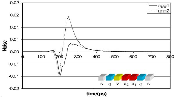
Figure 3: noises on the victim caused by two aggressors in a five-bit  $1000\mu\text{m}$ -long bus. The driver size is  $30\times$ , and the wire spacing is  $1.7\mu\text{m}$ .
