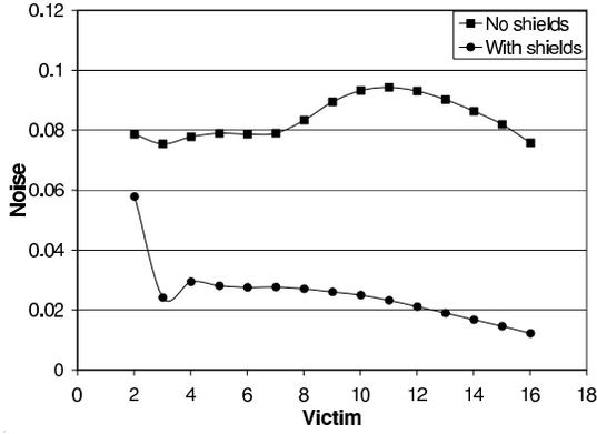
Figure 2: Noise in a sixteen-bit  $1000\mu\text{m}$ -long bus. The driver size is  $200\times$ , and the wire spacing is  $0.6\mu\text{m}$
