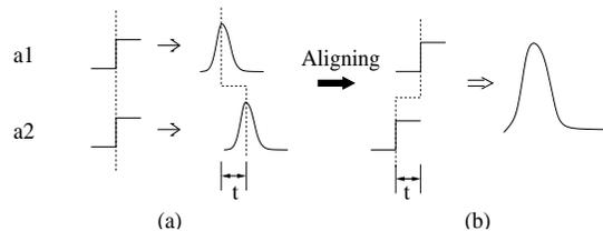
Figure 1: Alignment operation illustrated using two aggressors. (a) We simulate the interconnects with only one aggressor switching in each simulation, and find the skew  $t$  between noise peaks. (b) We simulate the interconnects with both aggressors switching. When their switching times are aligned by  $t$ , the overall noise due to the two aggressors is likely maximized [1].
